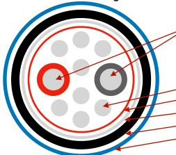
Central conductor: 2 conductors Copper OFC
